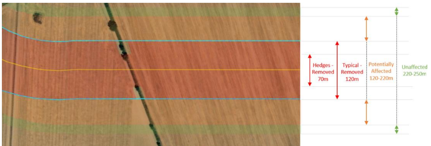
Image 4.13 Vegetation clearance requirements for underground cables
