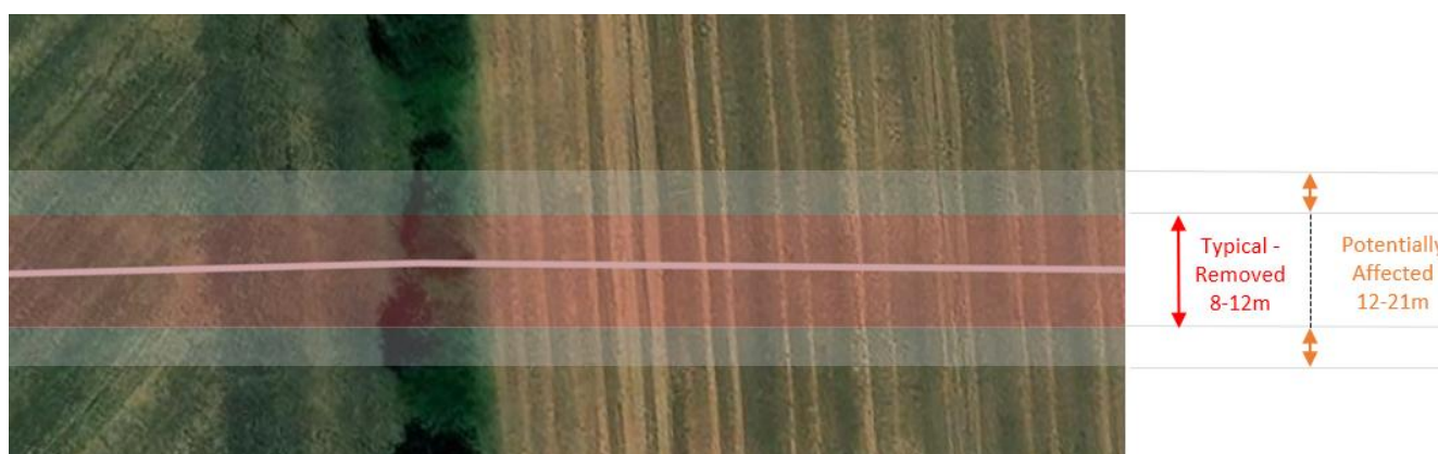
Image 4.4 Haul road vegetation clearance requirements
